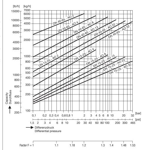
The max. differential pressure  $\Delta$  PMX of the equipment depends on the type of orifice (AO) used.
