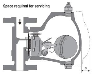
To remove the cover a withdrawal space S of 240/350 mm (depending on size) is required.
