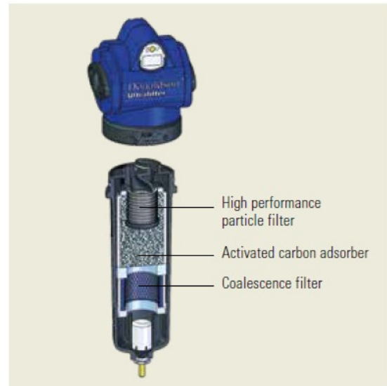
Cross-section of an Ultra-Filter with DF-T element
