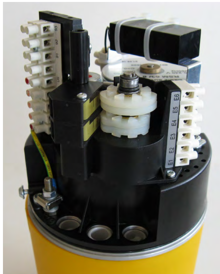
Fig. 12: 2EZ assembly on E07 actuator
