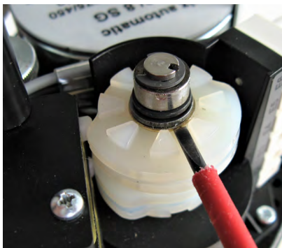
Fig. 14: Adjusting the switching cams
