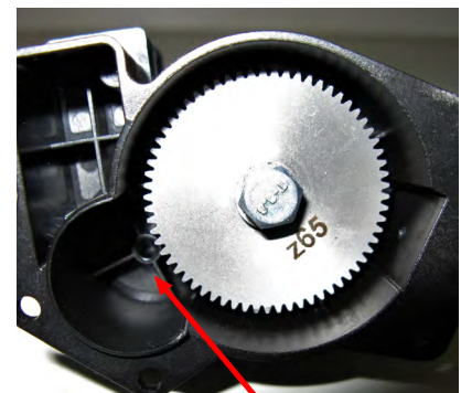
Fig. 10: Pinion fits here
