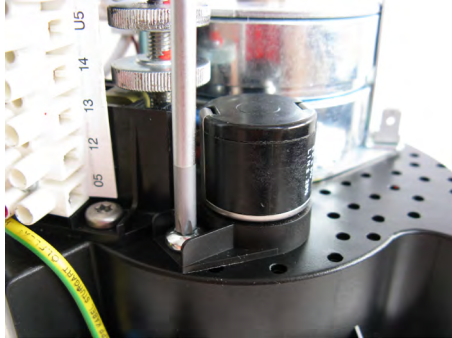
Fig. 6: Fixing the potentiometer
